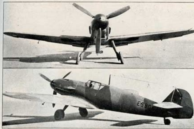
Two views of the Messerschmitt Me 109F Single-seat Fighter Monoplane (Daimler-Benz DB.601N engine).
